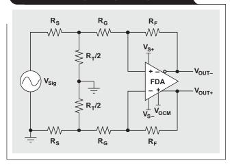
Figure 6. Equivalent SE bipolar input circuit
