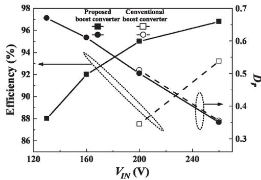
Fig. 9. Measured power efficiency and  $D_r$  versus  $V_{IN}$  for the proposed and conventional boost converters at  $V_O = 400$  V,  $f_s = 100$  kHz, and  $P_O = 300$  W.
