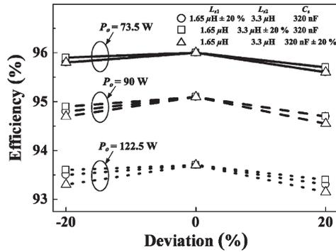
Fig. 6. Measured power efficiency for the proposed boost converter versus variation of circuit parameters from the designed values. Operating conditions:  $V_{IN} = 24$  V,  $V_O = 35$  V, and  $P_O = 73.5, 90,$  and  $122.5$  W.
