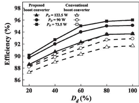
Fig. 7. Measured power efficiency versus  $D_d$  for the proposed boost converter in comparison with the conventional boost converter at  $P_O = 73.5, 90,$  and  $122.5$  W.
