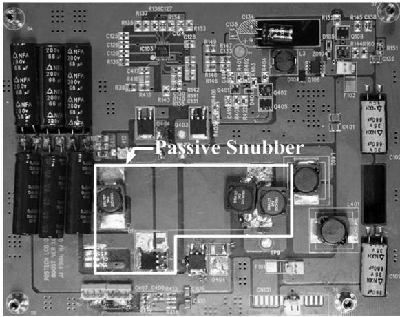
Fig. 3. Hardware circuit of the proposed boost converter.
