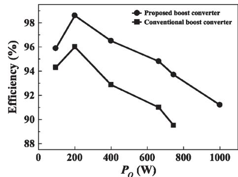
Fig. 8. Measured power efficiency versus  $P_O$  at  $V_{IN} = 85$  V,  $V_O = 160$  V, and  $f_s = 100$  kHz for the proposed boost converter in comparison with the conventional boost converter.
