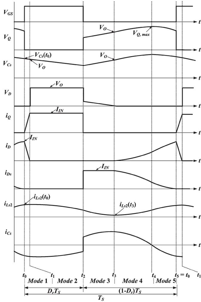
Fig. 2. Theoretical waveforms of the proposed boost converter.
