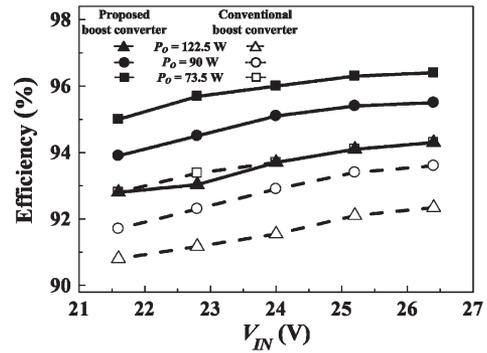
Fig. 5. Measured power efficiency versus  $V_{IN}$  ( $24 \text{ V} \pm 10\%$ ) for the proposed boost converter in comparison with the conventional boost converter at  $P_o = 73.5$ , 90, and 122.5 W.
