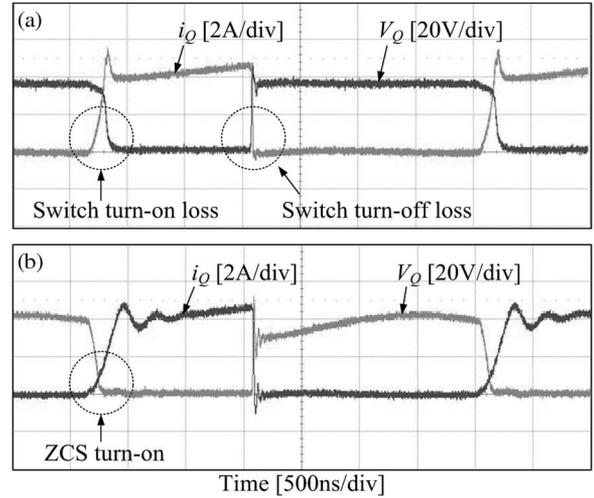
Fig. 4. Experimental current  $i_Q$  and voltage  $V_Q$  waveforms of switch  $Q$  at  $V_{IN} = 24$  V,  $V_o = 35$  V, and  $P_o = 90$  W: (a) conventional and (b) proposed boost converters.
