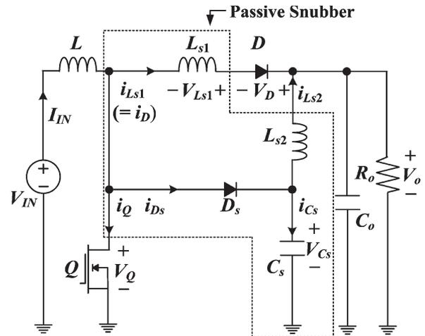
Fig. 1. Circuit diagram of the proposed boost converter. Its components are described in the text.
