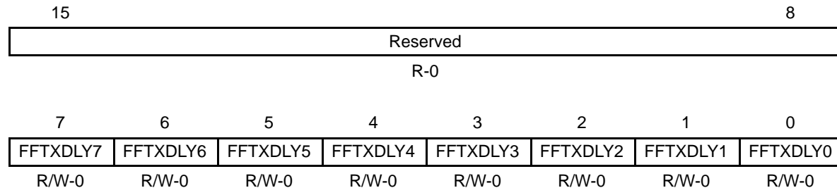
Figure 2–11. SPI FIFO Control (SPIFFCT) Register – Address 704Ch
