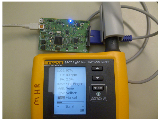
Figure 30. Fluke SPOT Light SpO2 Functional Tester Setup
