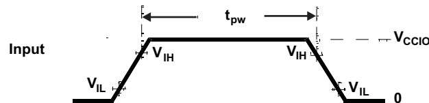
Figure 3-2. TTL-Level Inputs
