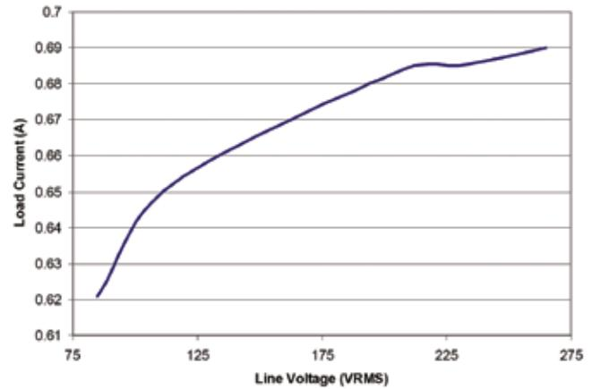
Load current as a function of line voltage. 10 Cree XLamp® 7090 XR-E, white, 700 mA LEDs connected in series was used for the load.
