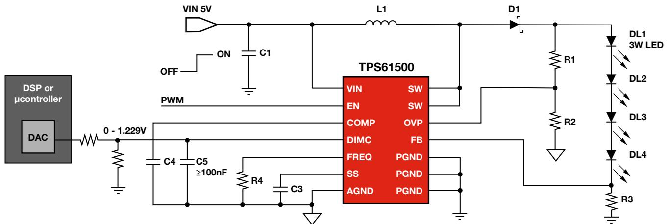
Analog Dimming by External DAC: Pure PWM Dimming Method
