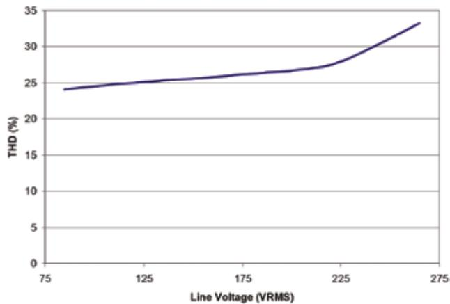
Total harmonic distortion as a function of line voltage. 10 Cree XLamp® 7090 XR-E, white, 700 mA LEDs connected in series was used for the load.
