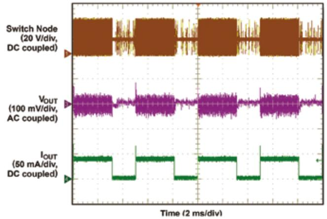
Mix Mode Dimming Current Linearity  $V_{IN} = 10.8\text{ V}$
