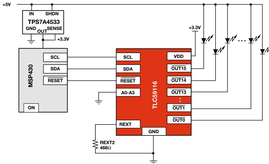
Figure 3. Analog Dimming/Blinking with a Load Switch
