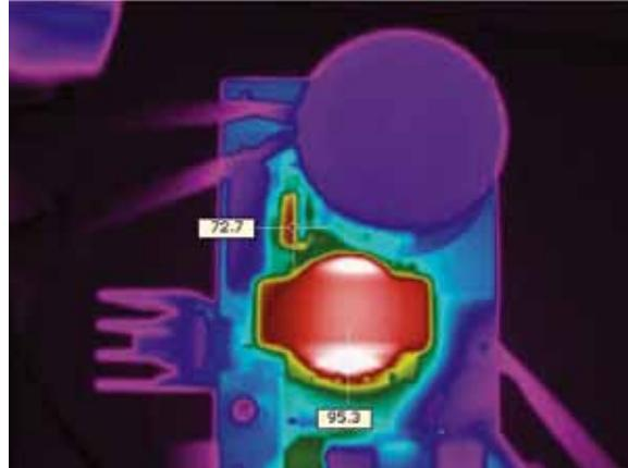
The image above shows a thermal image of the board. The ambient temperature was 26°C with no forced air flow. The input was 230 V<sub>AC</sub>.
