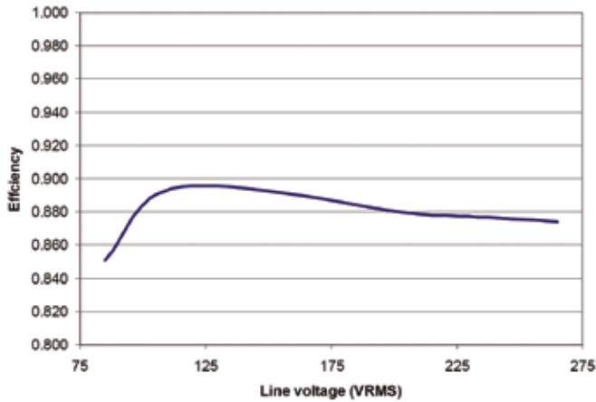
Efficiency as a function of line voltage. 10 Cree XLamp® 7090 XR-E, white, 700 mA LEDs connected in series was used for the load.
