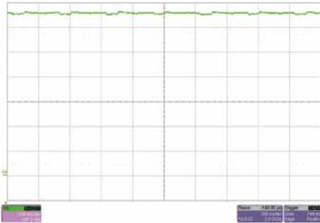
Output current with  $V_{IN} = 3\text{ V}$ .
