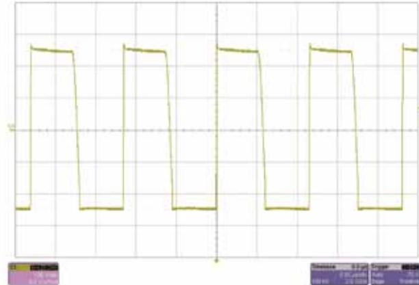
The image above shows the voltage on the anode of D1. The input was set to 250 V<sub>DC</sub>.
