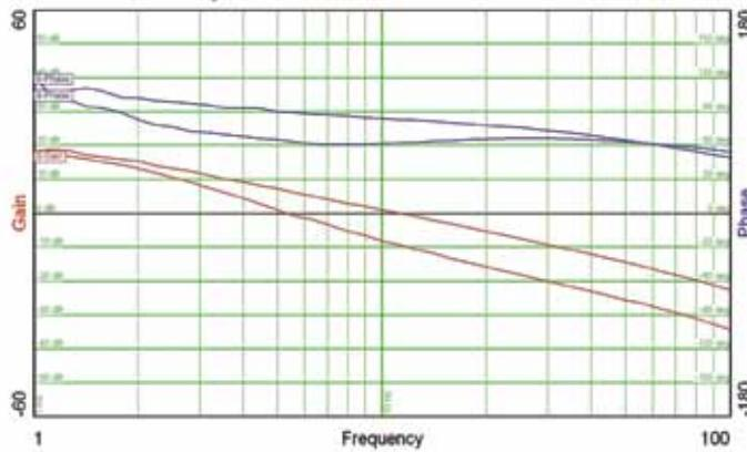
The frequency response of the feedback loop is shown in the plot above. The input was set to 220 V<sub>AC</sub>. The lower gain plot was taken with a 300 V output. The upper gain plot was taken with a 250 V output.
