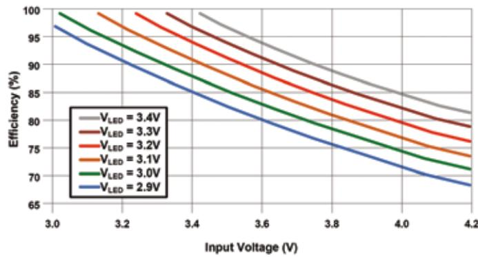
Figure 3 - LED Efficiency
