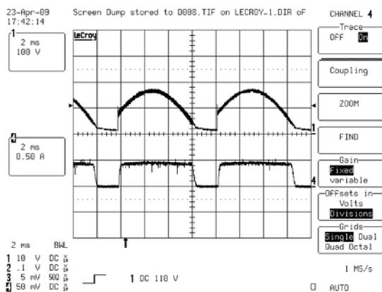
Line Current and Voltage – Dimmer at ~ Half Power Position
