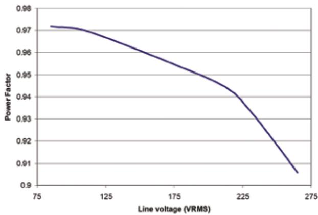
Power factor as a function of line voltage. 10 Cree XLamp® 7090 XR-E, white, 700 mA LEDs connected in series was used for the load.
