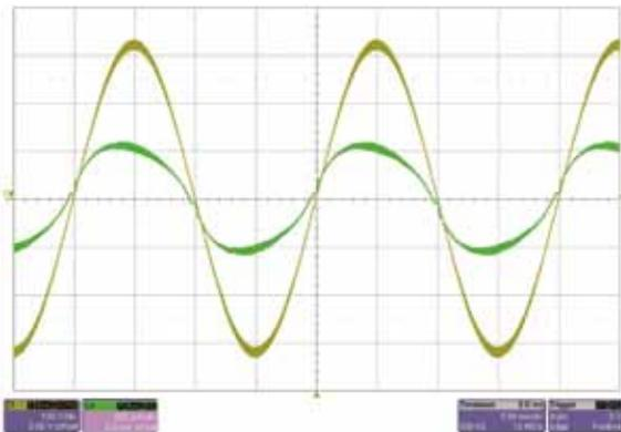
The image above shows the input voltage and current. The input voltage was 230 V<sub>AC</sub>.
