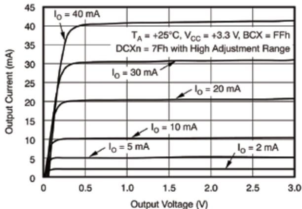
Dot-Correction (DC) Linearity (IOLCMax with Lower Range)
