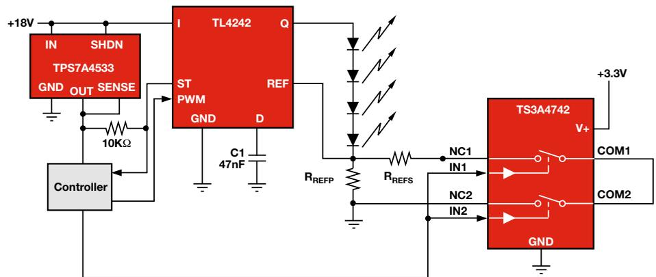
**Figure 3. Analog-Switch Brightness Control**
