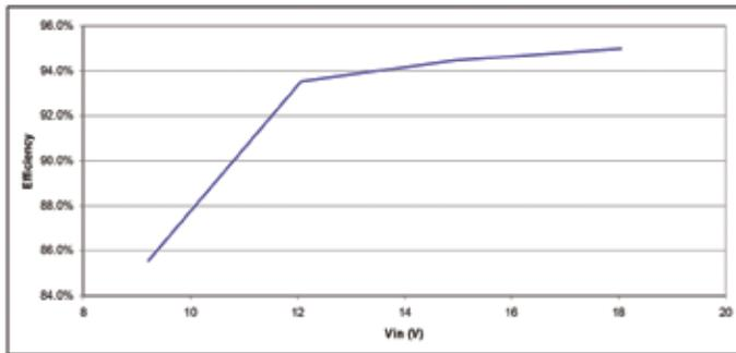
Total output current was 1.15 A, output voltage was 20 volts.
