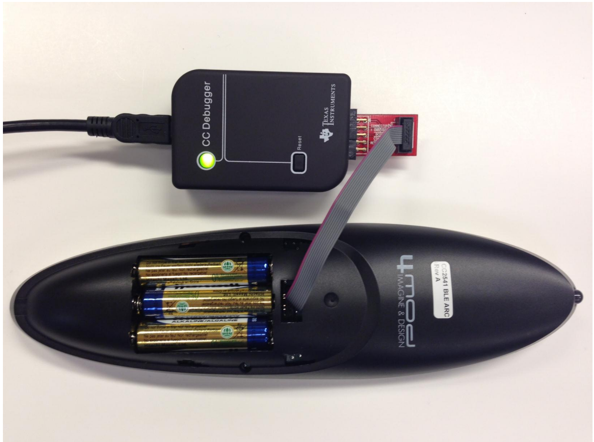
Figure 10 Advanced Remote Programming Setup
